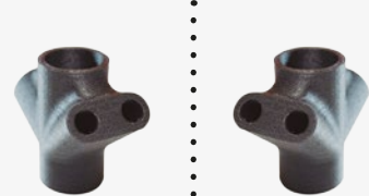
Mirror printing with 2 extruders
