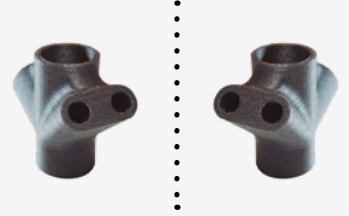
Mirror printing with 2 extruders
